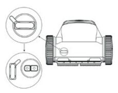
3 Connect to the power supply using the charger supplied.
