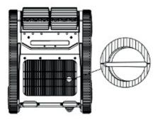
2 Remove the plug cover. When fully charged, cover the plug again.
